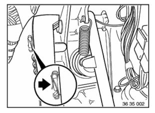
Remove locking clip for shaft pin of clutch cylinder.
